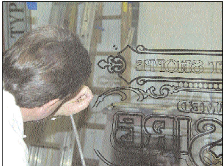
The second silk-screen is registered and the black outlines are printed. A little touch up is sometimes necessary.
