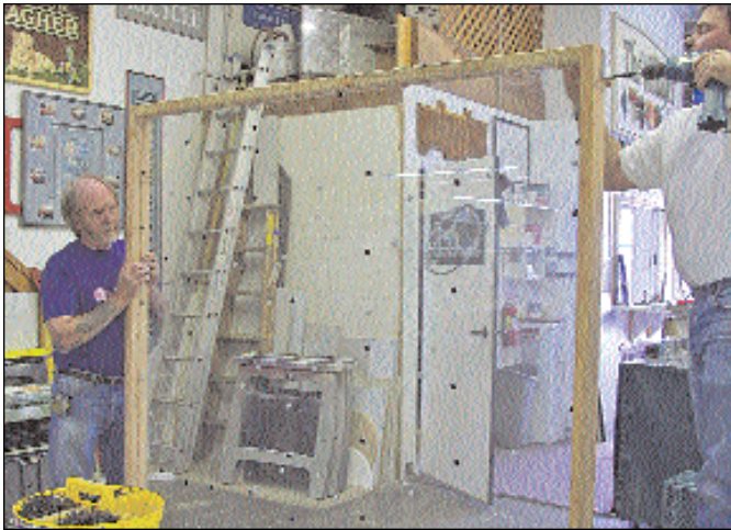
We had the luxury of working on the two large glass pieces in the shop. We are assembling the frame to hold the main piece of glass. The frame consists of dadoed 2x4 lumber, metal corner brackets and plywood legs to hold the glass vertical.
