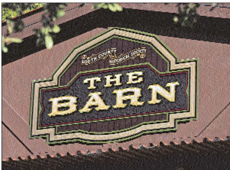
This sign was printed on the Gerber Edge and applied to a 4mm-cutout Dibond panel. Four tiles were necessary to facilitate this 4' x 5' print.
