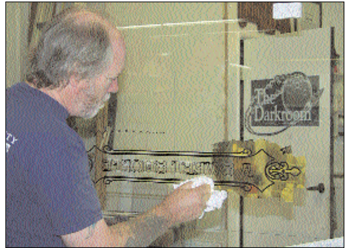
The pattern is registered, the first gold is laid where needed and the back-up paint is silk-screened. John Studden is removing the unwanted gold leaf.
