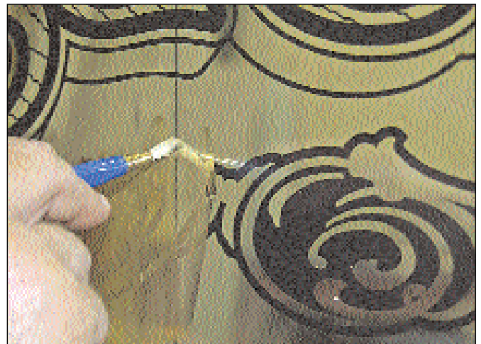
John is scratching away the hard edge of the 23-karat gold. The glass brush is made up of tiny glass hairs or rods and does a great job of removing areas of the gold leaf.
