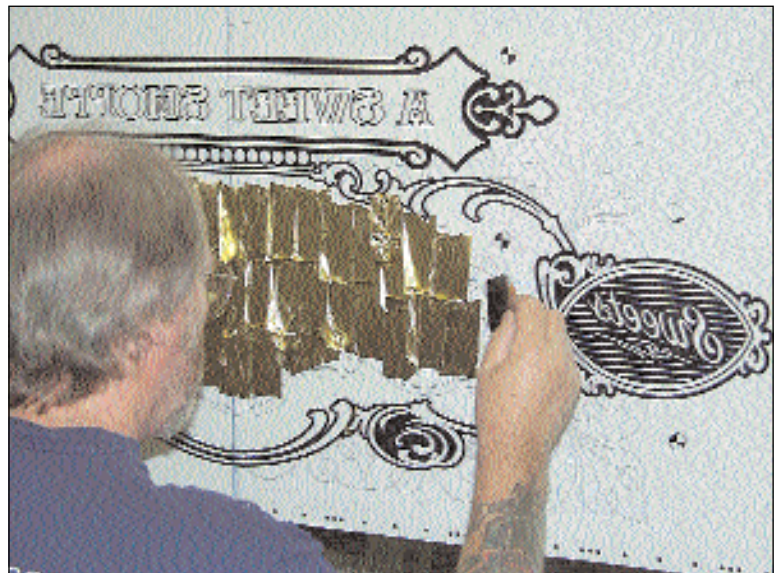
More 23-karat gold is applied with water size for the main copy.
