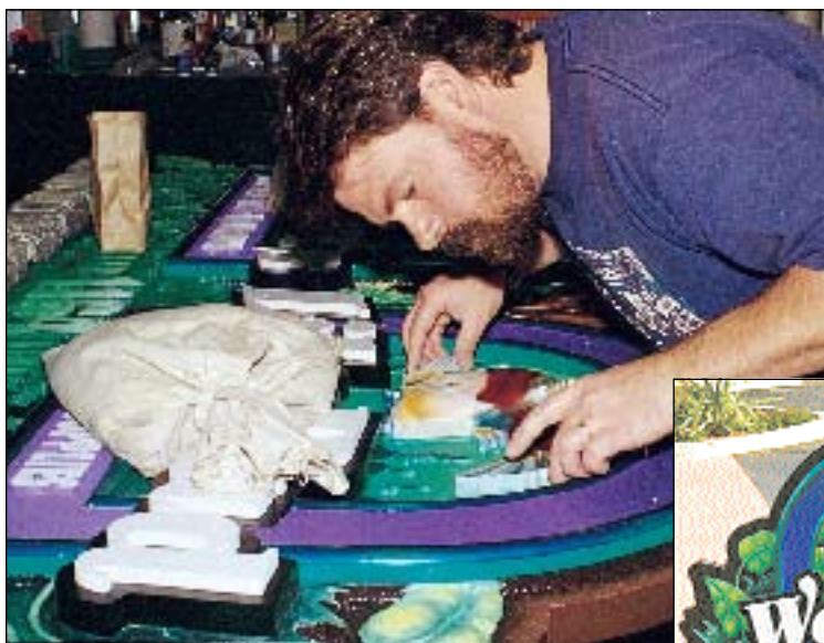
A two-part epoxy is used to apply larger appliques without the use of clamps. The aquarium was a little stubborn and needed some weight, hence the sand bag.
