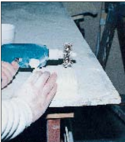
A wire brush chucked in a cordless drill created the stone. This is also great for wood grain.
