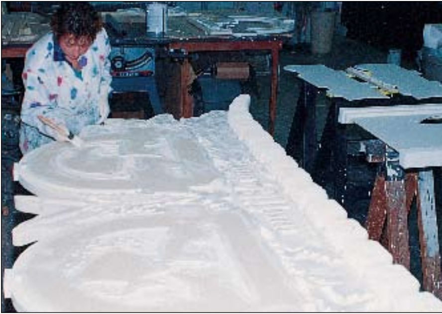
We give our HDU projects three good coats of oil-based primer.
