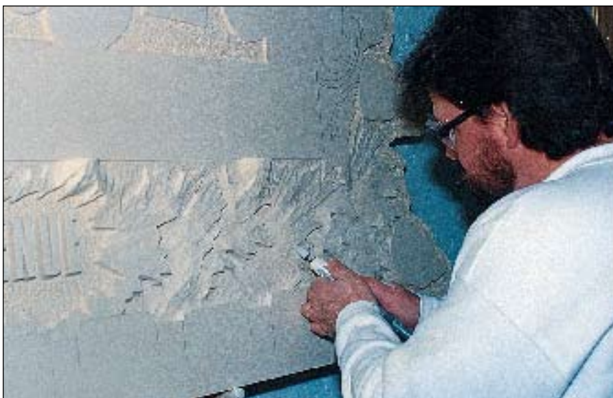
My worm-drive die grinder separates the organic elements in the background.
