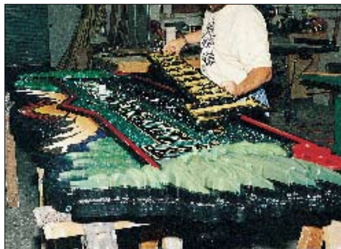
As you can see from this shot there were many layers on this sign. Using West System epoxy I attach the lettering.
