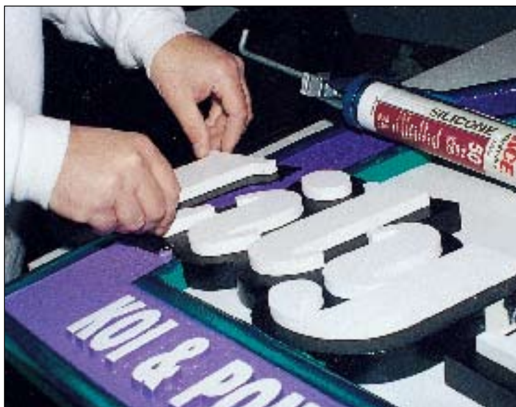
Letters cut from 1/2" Sintra are bonded to pre-painted HDU. Don't attempt to use silicone on the raw material; it is not recommended.
