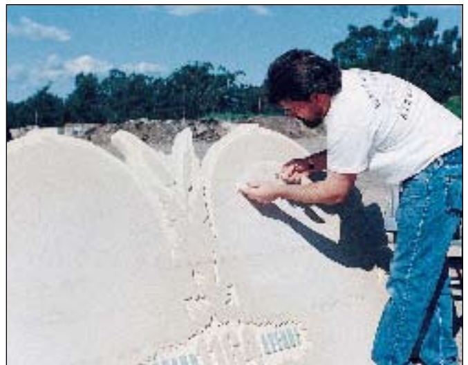
Note the shadows on the first stage of sandblasting. After removing the areas for the second level, the entire sign will be blasted another 1/4".
