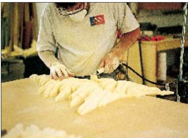
Here, I'm using a die grinder to sculpt the trees that will later be attached to the main sign.
