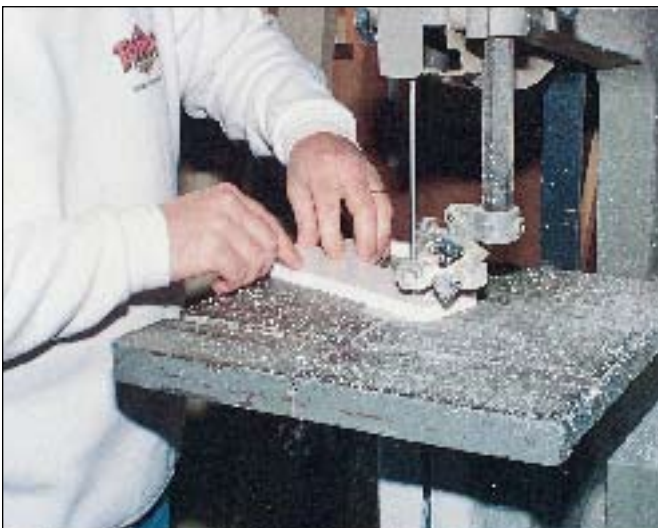
Using the band saw, the main copy is cut from 1/2" Sintra.
