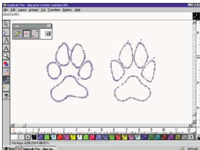
The left paw is scanned and the right paw is cleaned. I like to duplicate the item scanned, so I can compare as I clean up.
