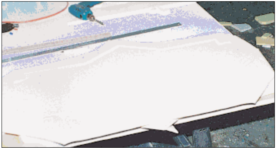
Sandblast resist has been applied and hand cut. Now it is ready to be sandblasted.
