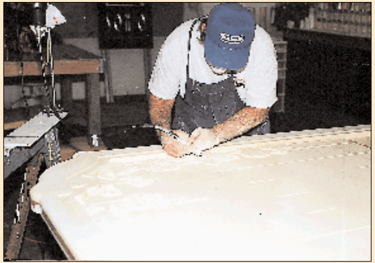
The router table was used for the initial profile on the grape leaves. Texture is added with a die grinder.
