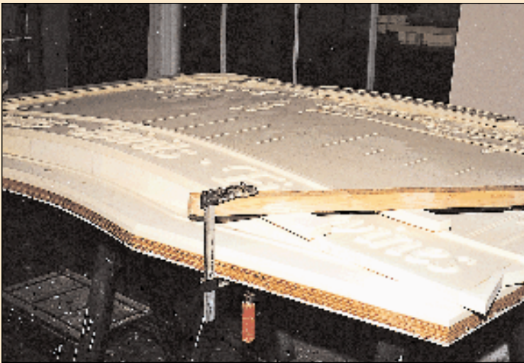
This banner could have been flat! Instead we cut a "bridge" profile to glue under the banner for added dimension. Clamps are employed to hold the shape until the epoxy dries.
