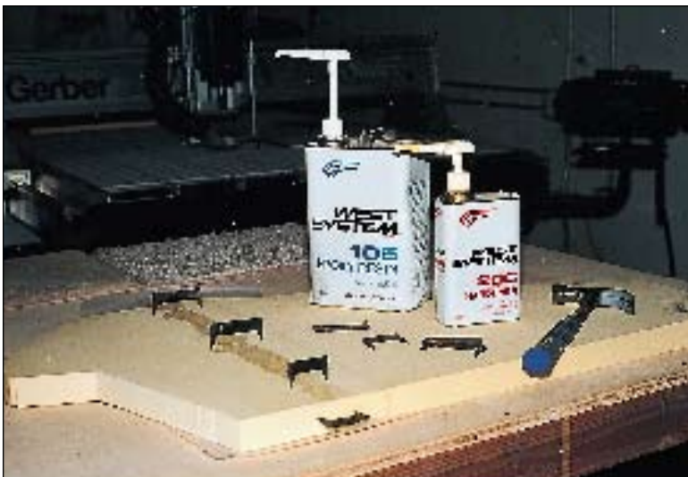
"Pinch dogs" are used to pull the edges together; the wax paper helps keep things cleaner.
